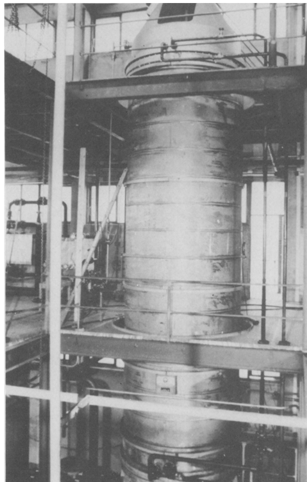
FIG. 25. Commercial molecular still.
